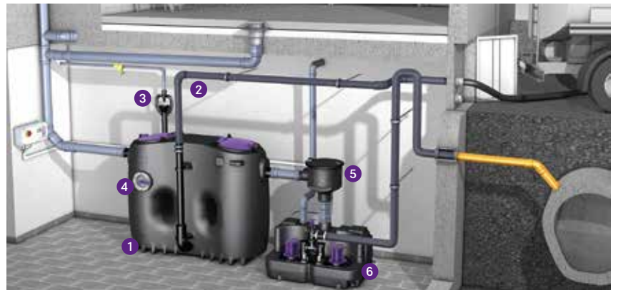
1 Grease separator EasyClean free Basic Direct 2 Odorless discharge is via a permanently installed discharge line 3 Refill inlet 4 Inspection window 5 Sampling chamber 6 Lifting station
